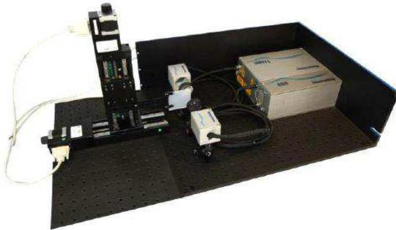
Figura 1b: Menlo Systems TERA K15 THz-TDS system with TERA image extension
