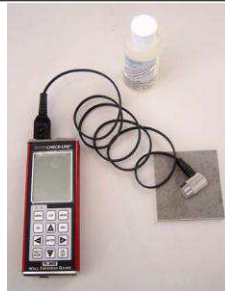
Fig. 8 - When only one structural side is available, an ultrasonic wall thickness gauge is used.
