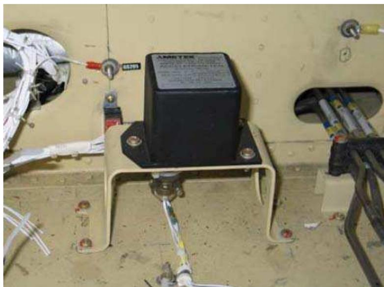
Figure 9. Acelerômetro de Fator de Carga (Taylor, 2007)
