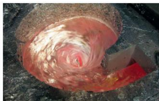
\ Sink vortex with molten metal on recirculation .
